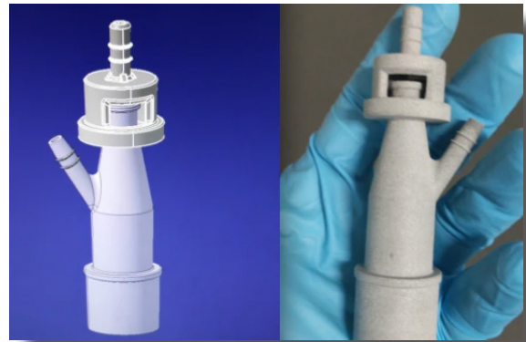
Image From Fast Company Article: These Good Samaritans with a 3D printer are saving lives by making new respirator valves for free
